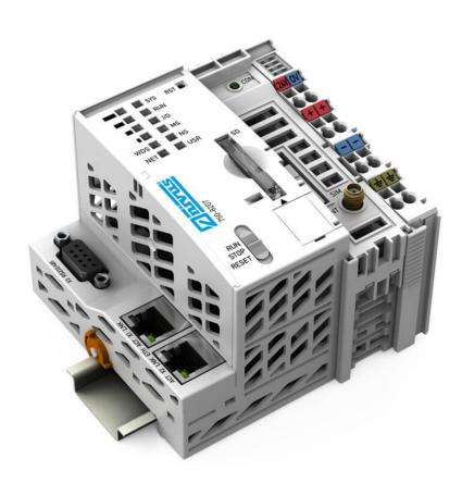
NivuLink Compact is an open and ready-to-operate solution for quick connection of measurement systems to the NIVUS Web Portal or other higher systems. Readings now can be saved centrally and represented in an easy-to-read manner.
